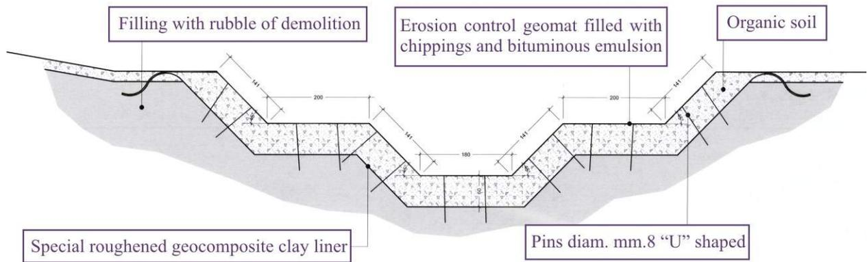
**Figure 7.** Cross section of the stream
