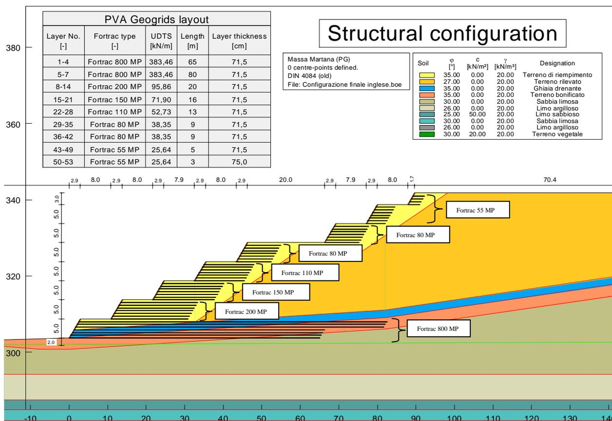
Figure 4. Structural configuration of most critical section in the reinforced embankment
